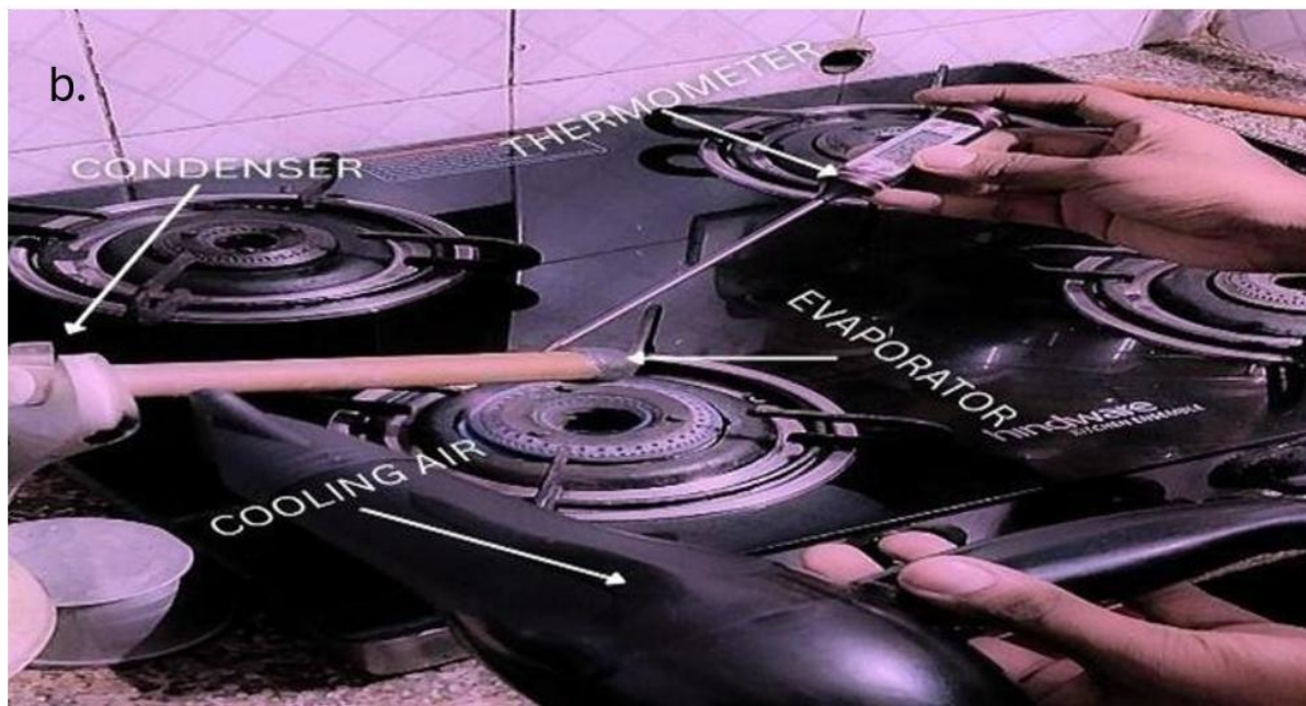
Fig. 2: (a) Schematic of the experimental setup, showing the evaporator (LPG burner), adiabatic section (cotton/aluminum-foil insulation), and condenser (hair dryer, cold-air mode), with the three thermometer locations and the direction of vapor flow and wick liquid return. (b) Photograph of the experimental setup: LPG burner at the evaporator end (right), cotton-and-aluminum-foil insulation on the adiabatic section (center), and a hair dryer providing cold-air forced convection at the condenser end (left).
