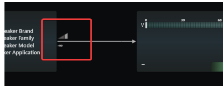
Figure 31 – +5V applied to the Level input has muted the output.
