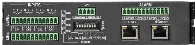
Figure 13 – Canali GPIO Section
